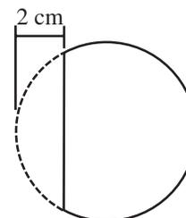
Figure 2.52 A high-speed tennis ball deforms when it hits a wall (Problem 2.12).
