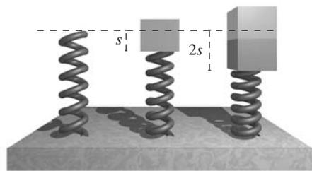
Figure 2.3 Compression of a spring is also a measure of force.
