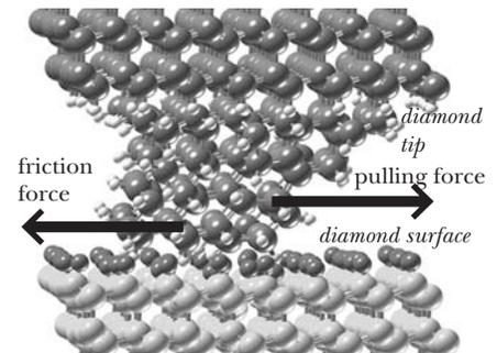
Figure 2.7 A computer simulation of sliding friction: a diamond tip is dragged along a diamond surface. Image courtesy of Judith A. Harrison, U.S. Naval Academy.
