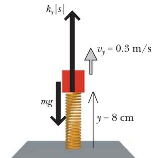
Figure 2.20 You compressed the spring, then released; the block heads upward with increasing speed, because the net force is nonzero and upward.
