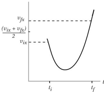
Figure 2.14  $v_x$  is not changing linearly with time. In this case the arithmetic average is much higher than the average value of  $v_x$ .
