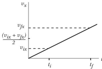
Figure 2.13  $v_x$  is changing linearly with time, so the arithmetic average is equal to
