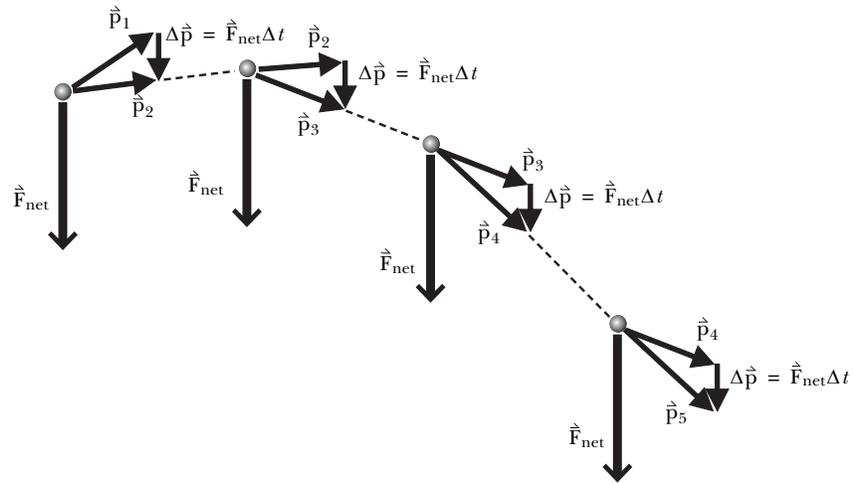
Graphical prediction of the motion of a ball, for three successive time steps.
