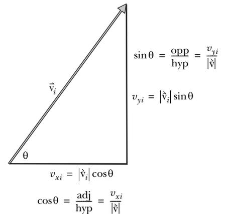
Figure 2.17 Converting speed and angle to velocity components.
