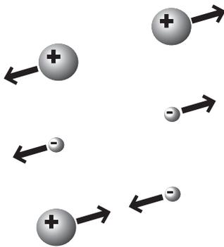
Figure 2.25 The electric force: protons repel each other; electrons repel each other; protons and electrons attract each other.
