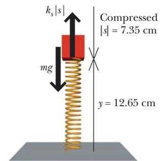
Figure 2.19 A block sits motionless on the spring. The net force must be zero.
