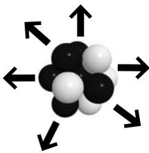
Figure 2.26 The strong force: the protons in the nucleus of an atom exert repulsive electric forces on each other, but the strong interaction holds the nucleus together despite this electric repulsion.
