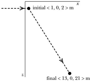
Figure 2.22 The  $x$  component of the momentum (and velocity) hardly changes, but the  $z$  component of momentum (and velocity) changes quickly from zero to some final value when the puck is hit.
