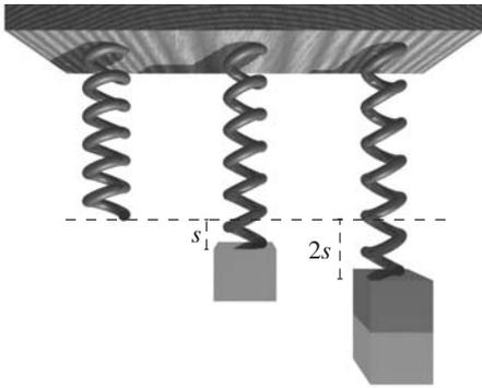
Figure 2.2 Stretching of a spring is a measure of force.
