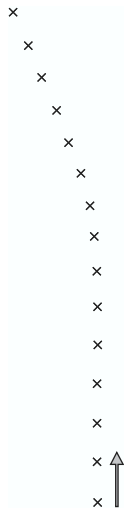
Figure 1.5 A proton moves through space, far from almost all other objects. The initial direction of the proton's motion is upward, as indicated by the arrow. The x's represent the position of the proton at equal time intervals.
