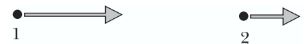
Figure 1.7 Two successive positions of a particle (indicated by a dot), with arrows indicating the velocity of the particle at each location. The shorter arrow indicates that the speed of the particle at location 2 is less than its speed at location 1.
