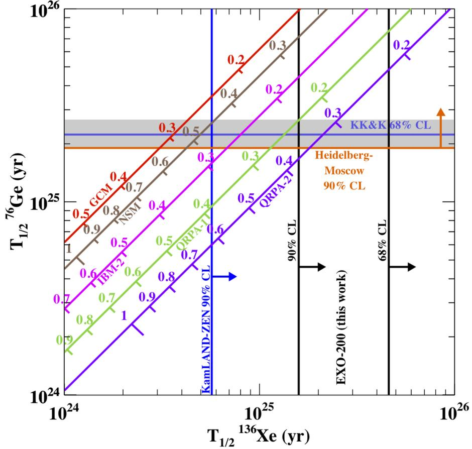
Figure 3: Relation between the  $T_{1/2}^{(0)}$  in  $^{76}\text{Ge}$  and  $^{136}\text{Xe}$  for different matrix element calculations. [8]
